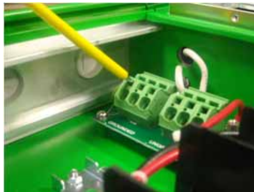
Figure 3-8 Releasing the Cage Clamp: step 1 (b)
